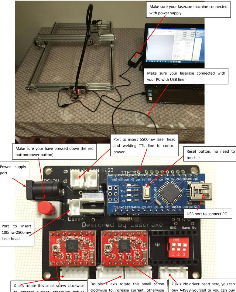
to increase current, otherwise reduce current, you can set direction in CNCC soft setting area. Double Y axis rotate this small screw clockwise to increase current, otherwise reduce current. This 2 port give opposite direction. You can set direction in CNCC soft setting area. Z axis. No driver insert here, you can buy A4988 yourself or you can buy from us directly. Same as X and Y axis
